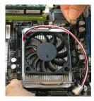
7. Connect the fan power cable from the mounted fan to the 3-pin fan power connector on the mainboard.
